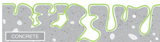
MICROSCOPIC CLOSE UP OF CONCRETE SURFACE USING A PENETRATING SEALER
